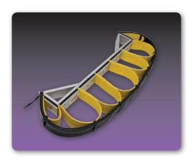
The **VB-Series High-Impact Sensing Bumpers** are designed to survive repeated crushing impacts that would destroy conventional bumpers. When deformed by contact or impact, they provide a signal in the form of an electrical contact closure. They are suitable for use on AGVs, mobile platforms, traveling conveyors, and other moving equipment or machinery. Sensitivity is uniform over the entire bumper surface, including any curved areas.
