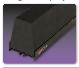
**SE-45 & SE-75 Sensing Bumpers** are designed for general-purpose, heavy-duty applications. When deformed by contact or impact, they provide a signal in the form of an electrical contact closure. At the same time, the large, compliant surface and substantial overtravel cushioning helps protect personnel and equipment from injury or damage. Operating force is 20 lbs. nominal.
